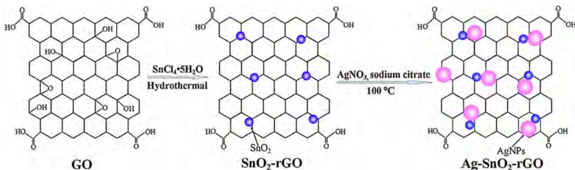
Scheme 1. Schematic illustration of the synthesis of AgNPs-SnO 2 -rGO hybrids.
